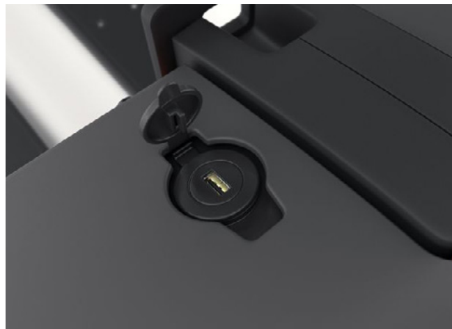
5V USB outlet for simple charging of smart phone, tablet or other external equipment.
