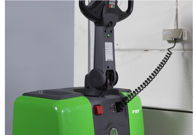
The control panel includes a pull-out power lead for the built-in battery charger.
