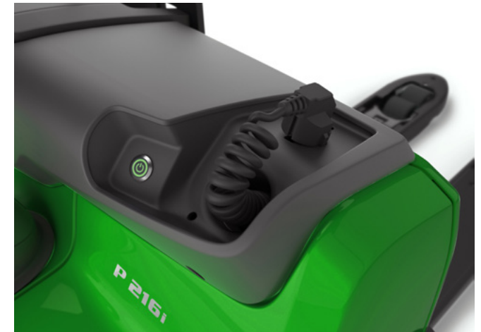
Easy and fast charging with the built-in charger for more energy efficiency (external charger also available).
