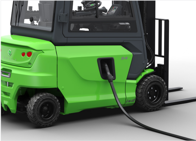
The conventional model can be equipped with lithium-ion battery. An easy access to battery plug on lateral door allows for easy, quick and safe opportunity charging.
