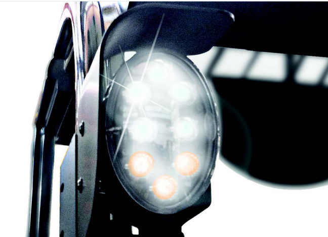
Powerful and efficient LED working lights allow work to continue in unlit areas or at night.
