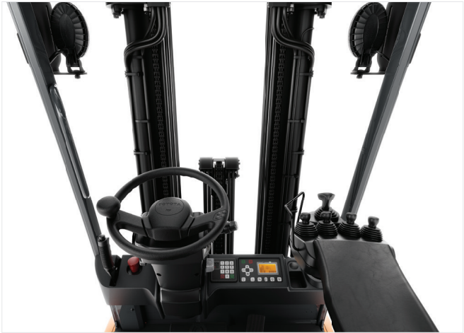
Excellent visibility through the mast with low dashboard including built-in display with essential driver information and functions.
