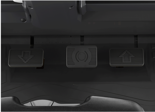
Different pedal layouts are available to fit drivers' preferences. Double accelerator pedals allow the operator to change driving direction with the feet.
