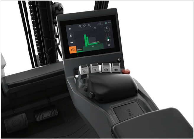
Display & lever options have been designed with the operator in mind for optimal comfort and productivity. The colour touchscreen display is both intuitive and interactive showing essential parameters and controls.
