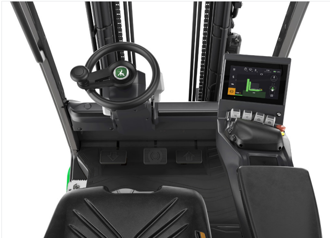
Increasing driver comfort with the new tiltable and telescopic steering column, which enhance the space for the operator.
